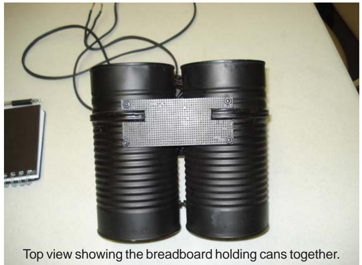
Top view showing the breadboard holding cans together.
